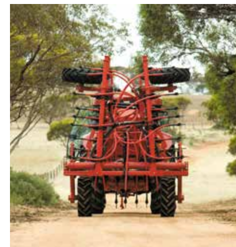
Folded 3m transport width with mounted airseeder.
