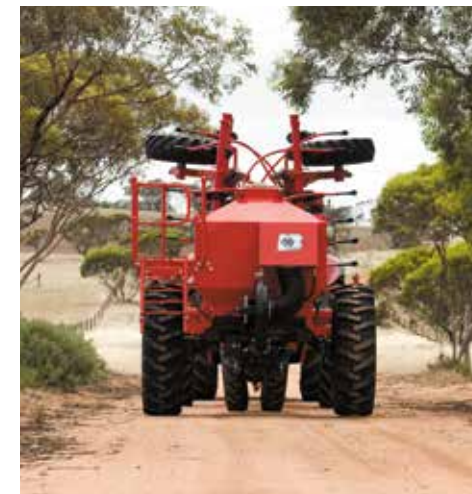
Folded 3m transport width with tow-behind airseeder.
