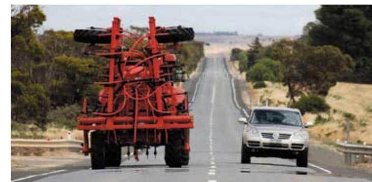
Clever wing fold and 2m wide track enable safer transport between sites.
